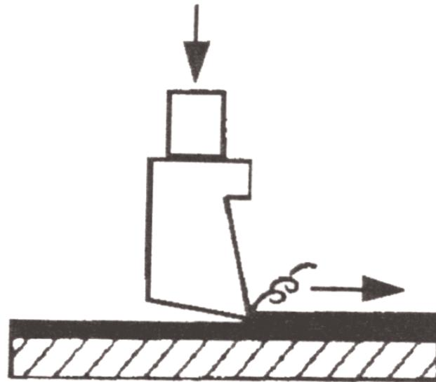
*Scratch Tool: Test Tip acc. to Clemen*
