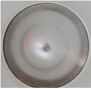
Light of luminous punch shining through crack
